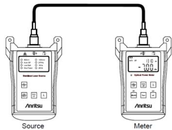
**Figure 3 Checking Output Power**
