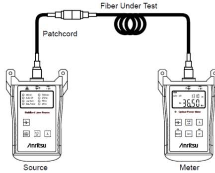
**Figure 4 Optical Loss Measurement Setup**
